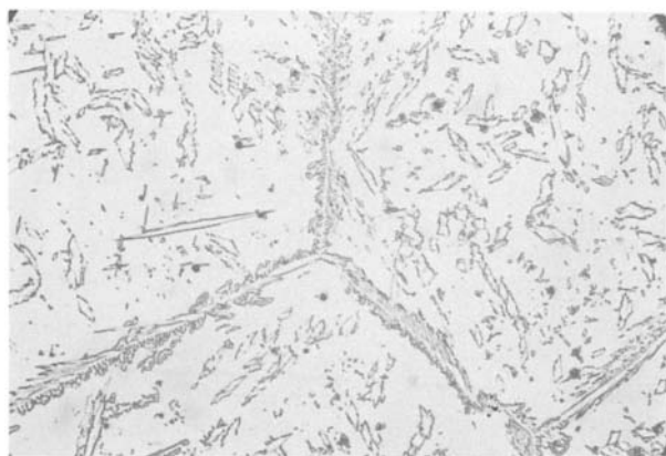
Figure 1 Light optical micrograph of the 26Cr-5Ni alloy. Solution treatment (1300°C, 30 min), isothermal transformation (800°C, 5 min) and air cooling. Magnification \times 150 .
