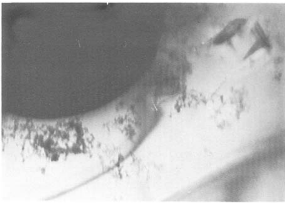
Figure 5 Transmission electron micrograph showing precipitation of particles on dislocations. Magnification \times 53000 .
