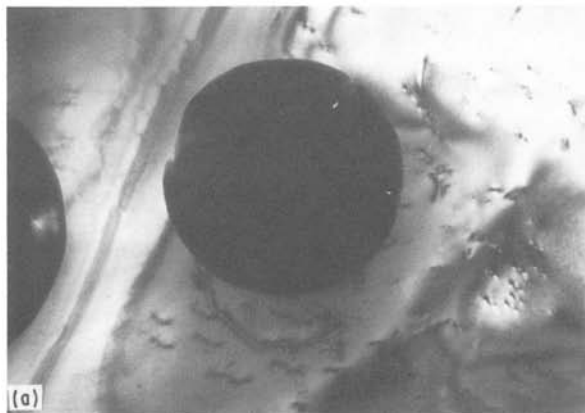
Figure 4 Transmission electron micrographs showing weld metal inclusions surrounded by dislocations and dislocation loops. Magnification (a) \times 28\,000 (b) \times 42\,500 .
